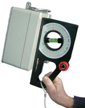
Rotate VIKING+ around its horizontal axis until the inclinometer's bubble reaches its central position between the two marks, at which point the radar is tilted properly and nut 2 can be tightened again.
