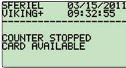
The "CARD AVAILABLE" display indicates that it is important to insert or remove the SD card only when the counter is off. This prevents the risk of corrupting the stored data if the SD card is removed by mistake while the counter is still recording.
