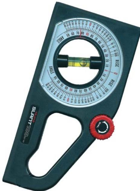
From now on, the DIAL button should not be touched again and the inclinometer is to be used as a simple spirit level. Nut 2 of the mounting bracket must be loosened and the inclinometer pressed against the front panel of VIKING+, as shown on the next page.
